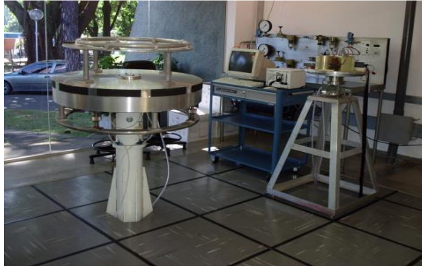
Figure 1. INPE 3D and 1D Satellite Attitude Control System Simulators.
